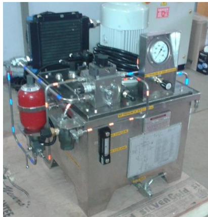
Hydraulic Power Unit with Water Glycol compatibility
